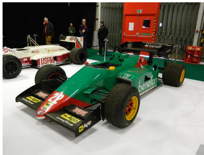
Alfa Romeo 185T, 6 speed 1500cc turbo, 750bhp as driven by Riccardo Patrese
